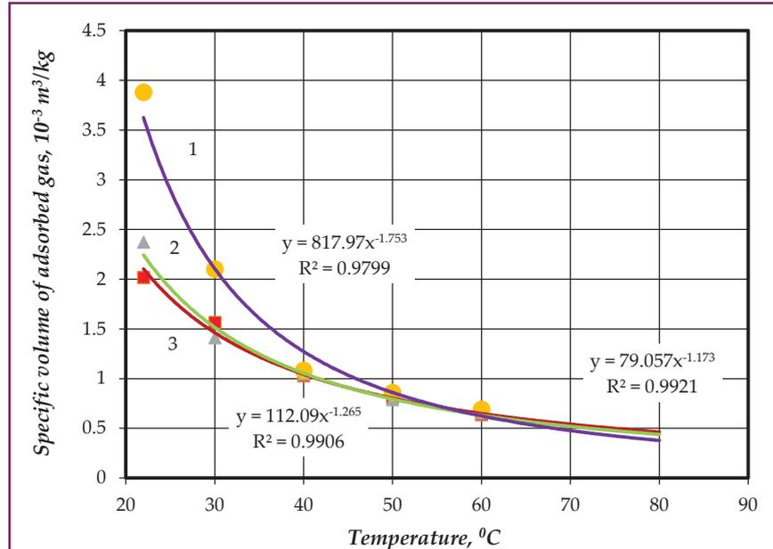
**Fig.3. Graphical dependences of adsorbed gas content from temperature (adsorption isobar) for different pressures (model with permeability – 9.7mD): 1 – 20 MPa; 2 – 10 MPa; 3 – 8 MPa**
