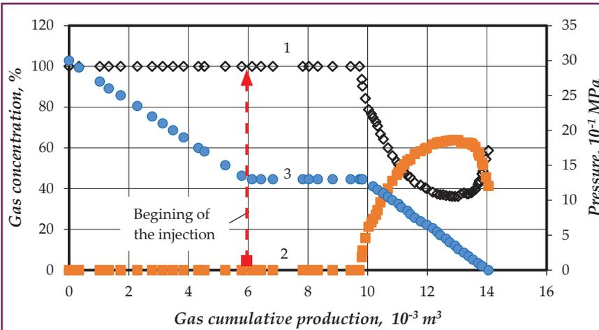
**Fig.5. The dynamics of pressure and components concentration in produced gas during the implementation of the method of full voidage replacement at the pressure of 0.4 from initial pressure:**
