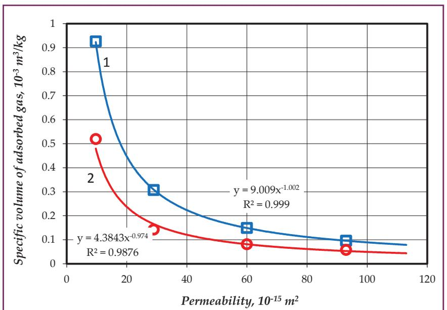
**Fig.2. Dependences of specific volume of adsorbed gas on the model permeability for different values of temperature under the pressure of 3 MPa: 1 – 40 °C; 2 – 60 °C.**
