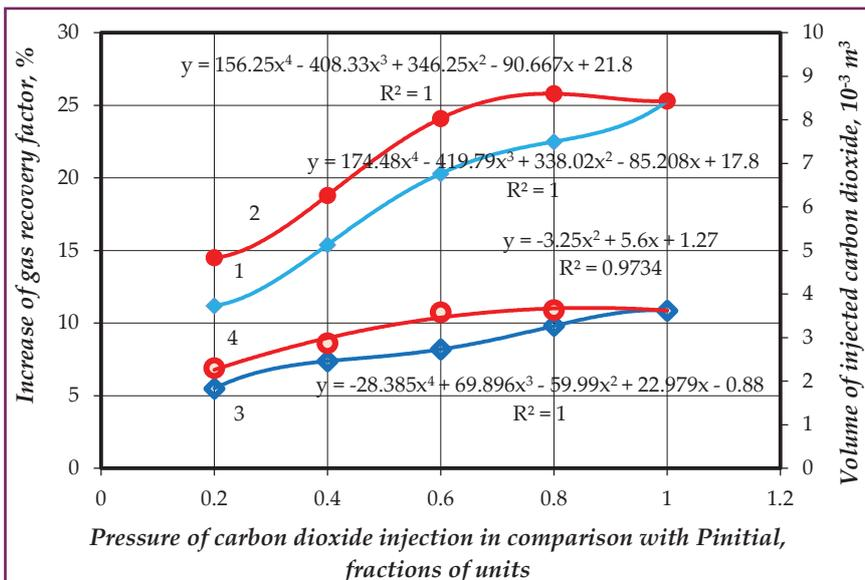
**Fig.9. Graphic interpretation of experiment results in methane displacement by using carbon dioxide**
