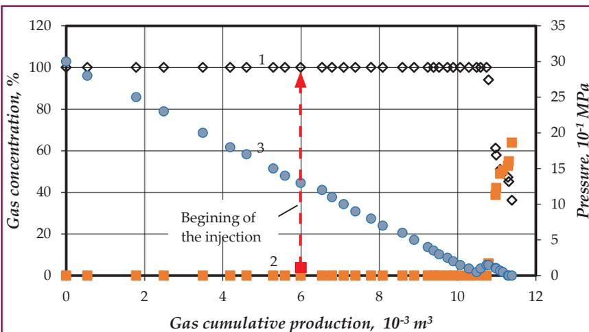
**Fig.7. The dynamics of pressure and components concentration in produced gas during the implementation of the method of partial voidage replacement at the pressure of 0.4 from the initial pressure:**
