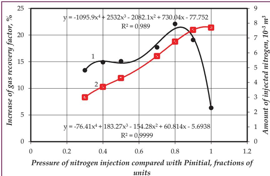
**Fig.8. Graphic interpretation of experimental data on methane displacement by nitrogen**
