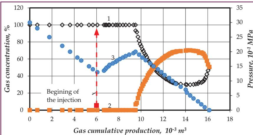
**Fig.6. The dynamics of pressure and components concentration in produced gas during the implementation of the method of higher voidage replacement at the pressure of 0.4 from the initial pressure from initial pressure:**
