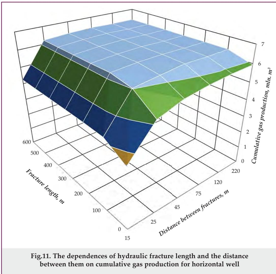
**Fig.11. The dependences of hydraulic fracture length and the distance between them on cumulative gas production for horizontal well**
