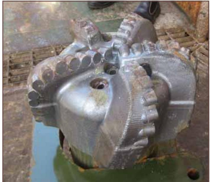
**Fig.2 8 1/2" PDC bit used in the third open drilling process**
