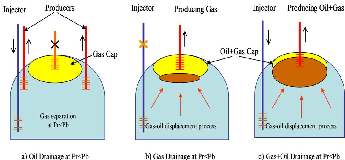
**Fig.2. Scheme of producing Bach Ho basement reservoir at pressure lower than bubble point**
