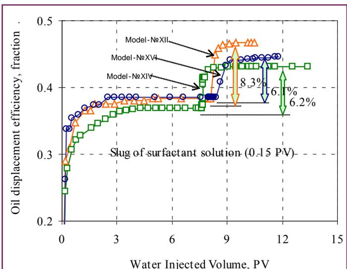
**Fig.3. Oil displacement behavior at water/polymer flooding on layering core models of BH Low Miocene reservoir**
