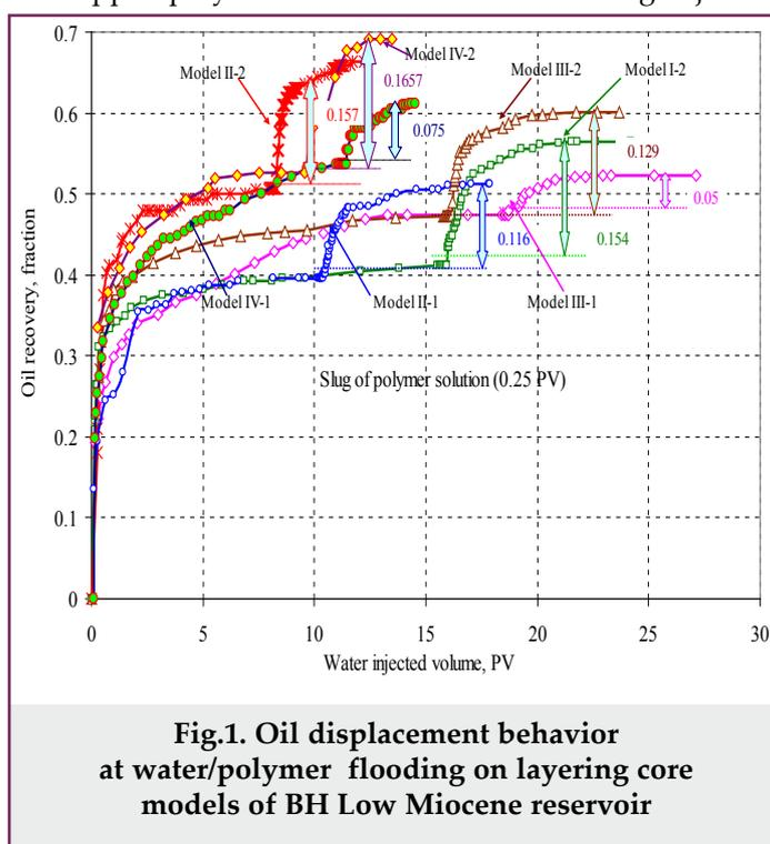
regime of 0.25 pore volume showed that the average increment of oil recovery is 0.121. Oil displacement behaviors were identical for all experiments and sharp increase in oil recovery right after renewing water injection was observed [3].
