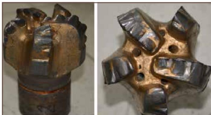
Fig. 12. Experiment PDC bit with cutting angle 0°
