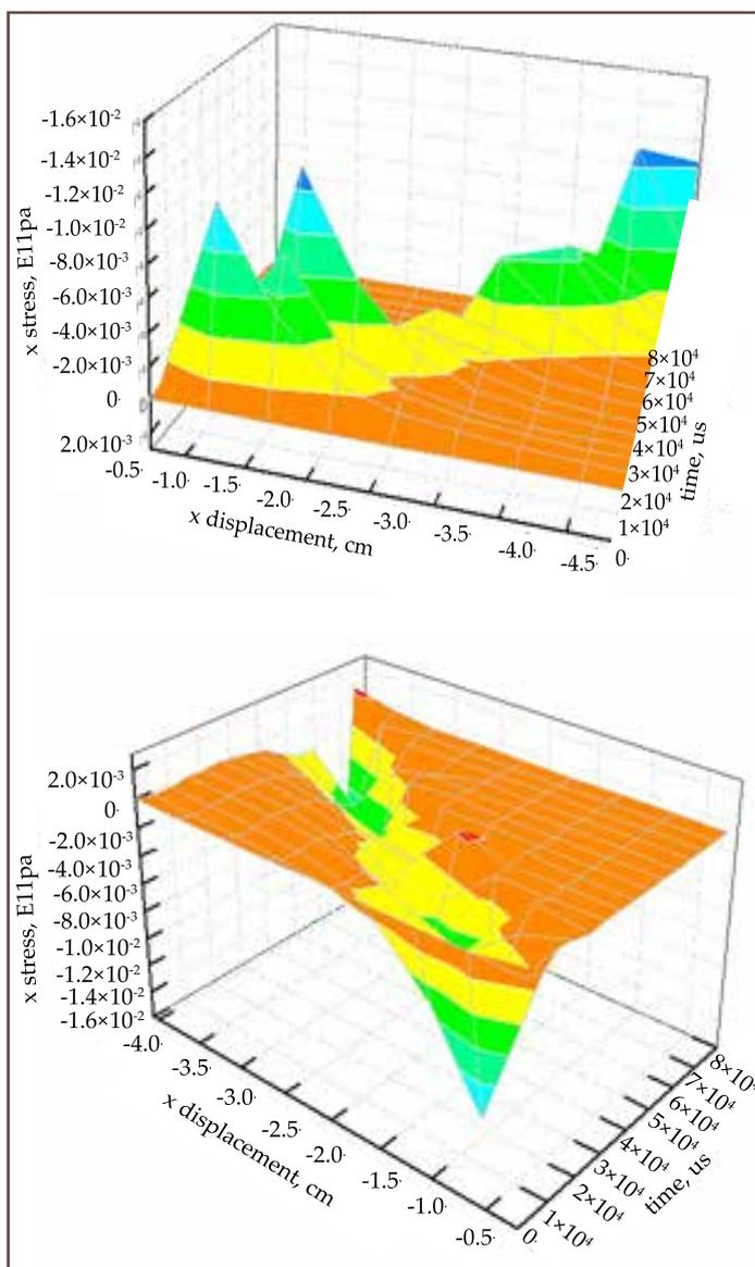
Fig.5. 3D-visualization of time-position-stress in different x-position of granite
