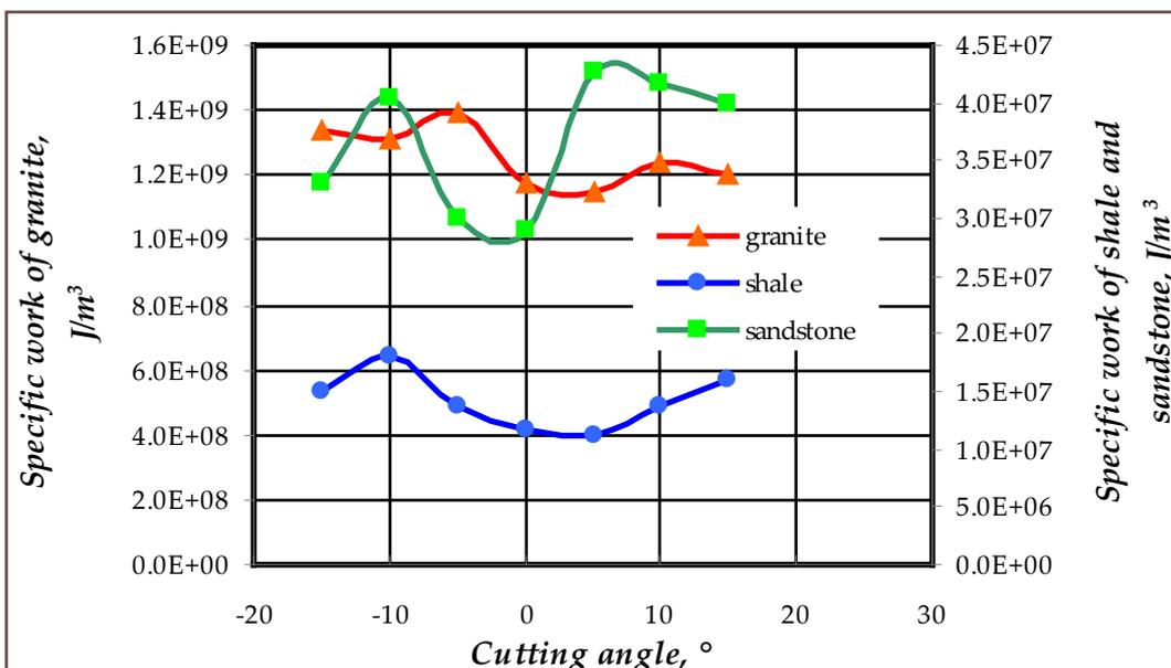
Fig.10. Relation curve of specific work and cutting angle
