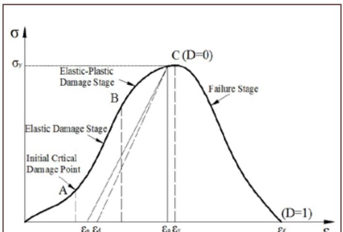
Fig.3. Stress-strain curve of sandstone somewhere
