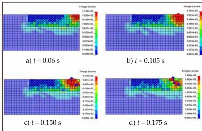
**Fig.6. Von Mises equivalent stress at different time of granite**
