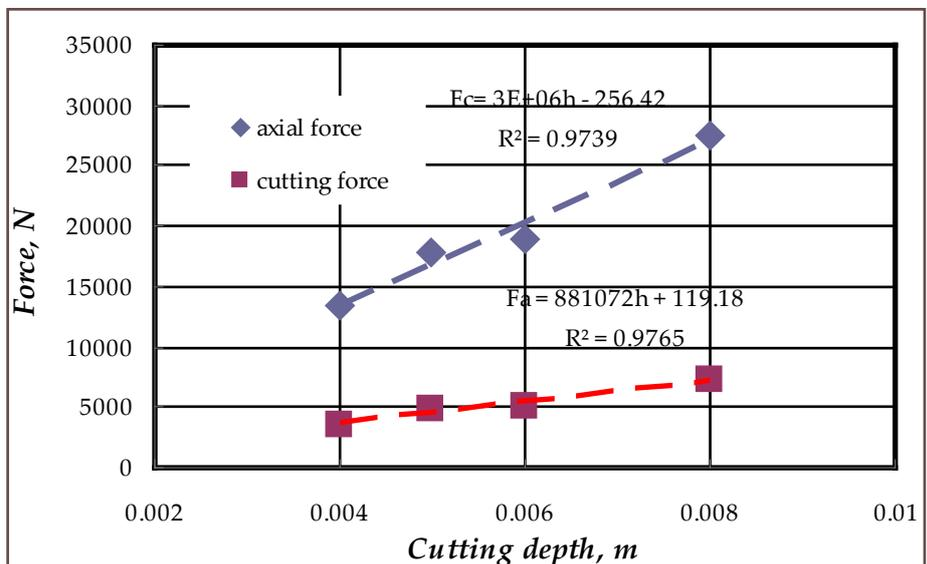
**Fig.8. Relation curve of force and cutting depth**
