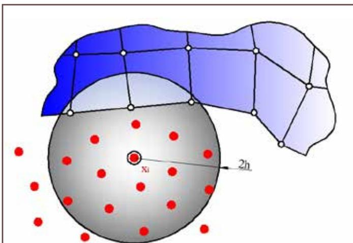
Fig.2. Contact sketch of SPH particles and FE nodes
