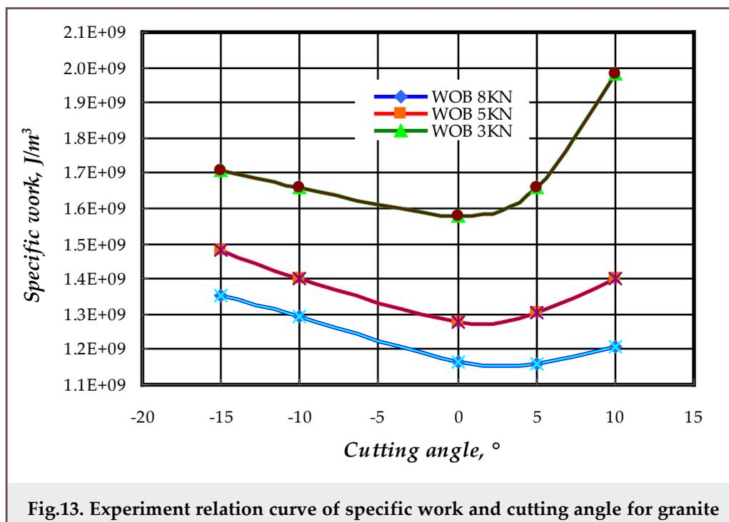
Fig.13. Experiment relation curve of specific work and cutting angle for granite
