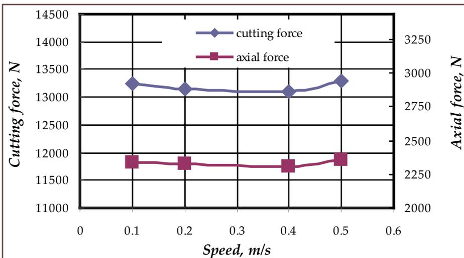
Fig.9. Relation curve of force and cutting speed
