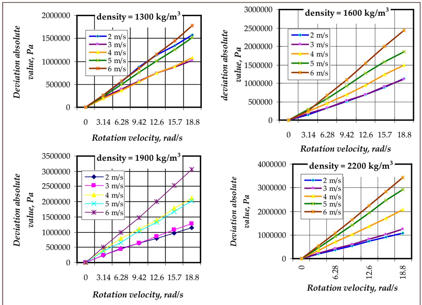
Fig.7. Friction pressure loss deviation absolute value in rotating drill string
