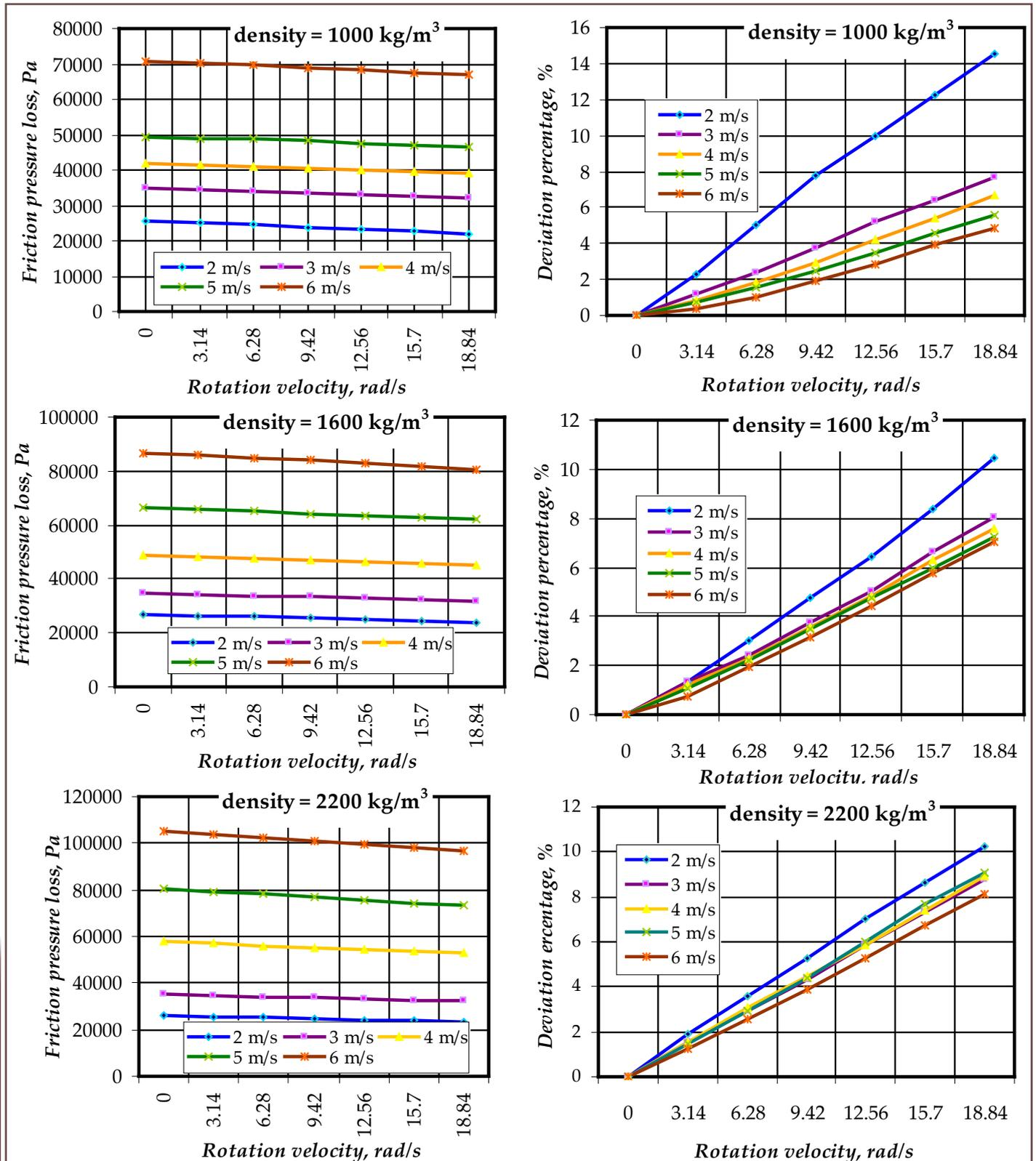
Fig.6. Friction pressure loss and deviation percentage in rotating drill string
