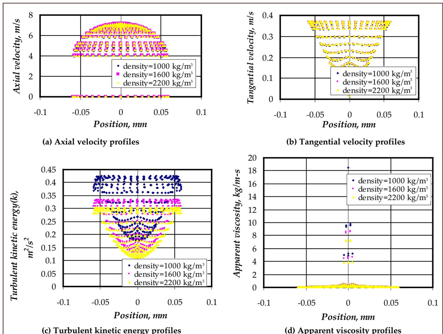
Fig.5. Impact of fluid density on helical flow field (rotation velocity =  $18.84 \text{ rad/s}$ , axial velocity =  $4 \text{ m/s}$ )
