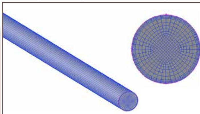
Fig.1. Geometric model in drill string
