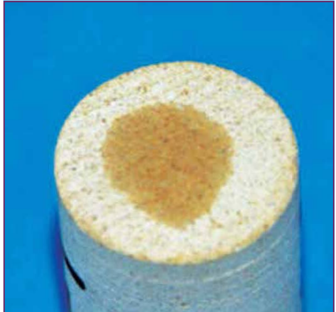
Fig.6. Shape of fracturing filtrate dripped onto the surface of tight sandstone core after 30 s
