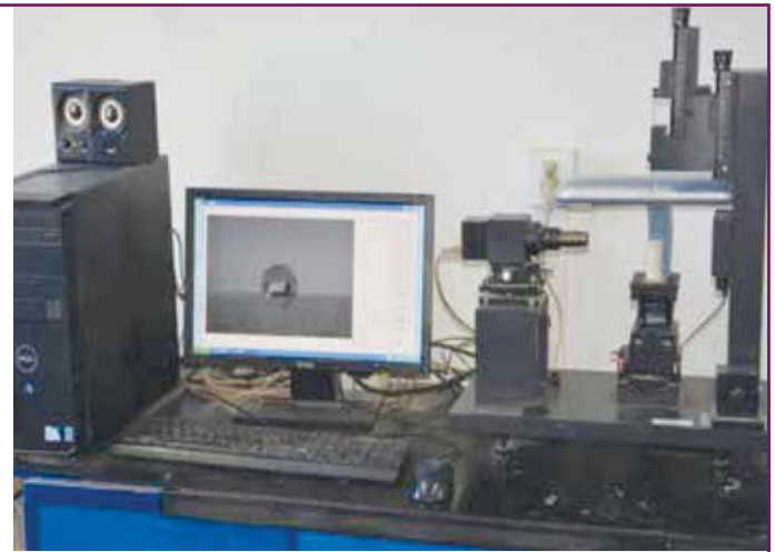
(b) Experimental set-up of solid-liquid contact angle measurement
