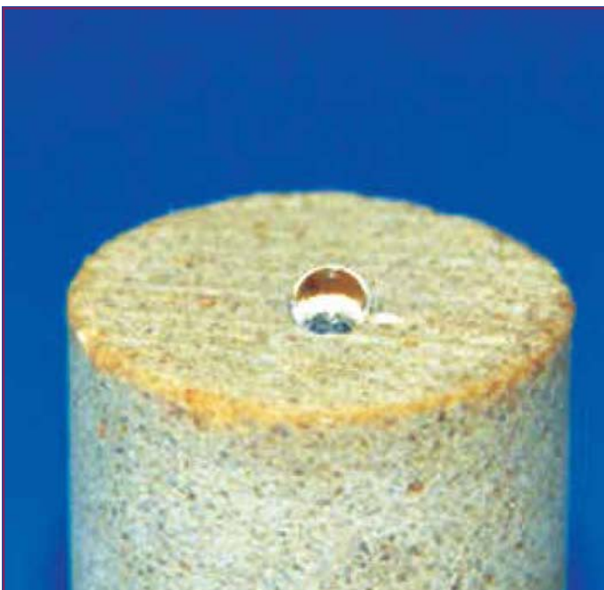
Fig.7. Shape of fracturing filtrate immediately after dripped onto the surface of tight sandstone core treated by 1% FCS
