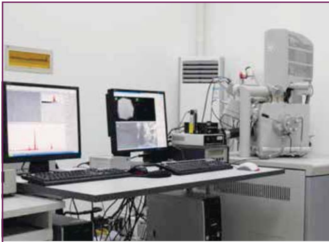
(a) Experimental set-up of energy spectrum analysis and surface appearance of cores
