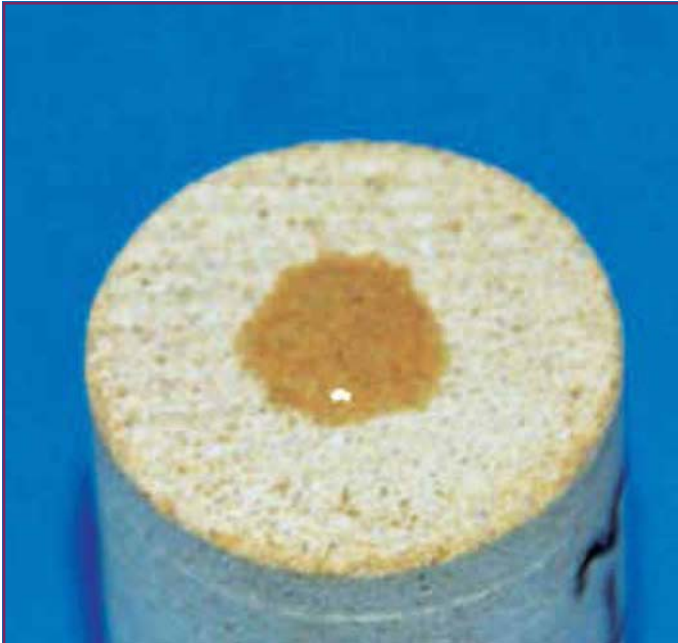
Fig.5. Shape of fracturing filtrate immediately after dripped onto the surface of tight sandstone core
