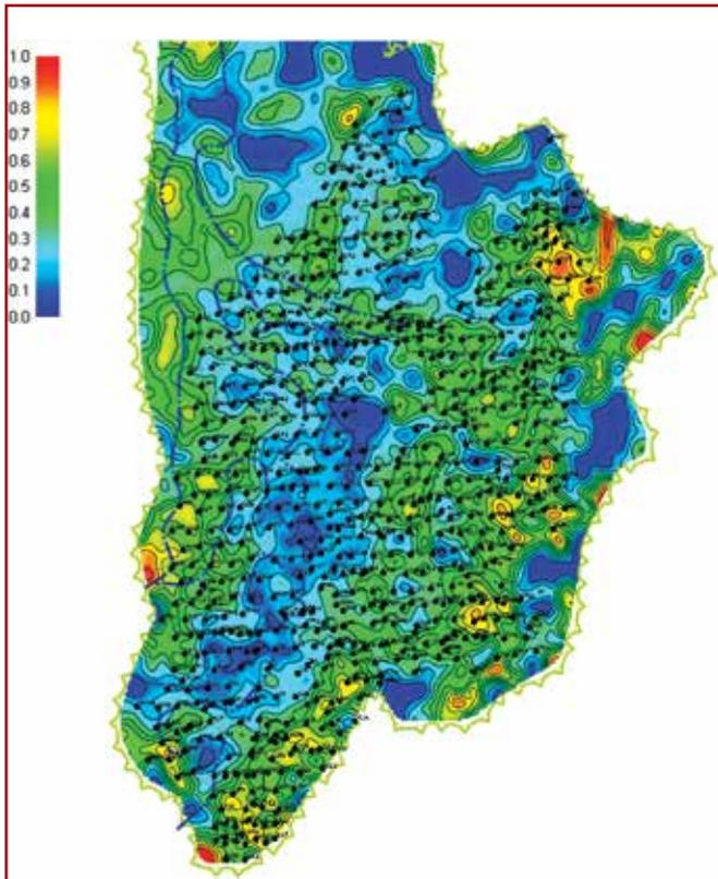
Fig.5. Net-to-gross-ratio map in oil-bearing strata BS 10-2/3
