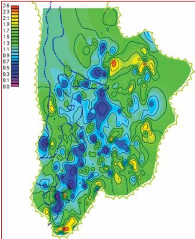
Fig.4. Permeability (log scale) map of oil-bearing strata BS 10-2/3
