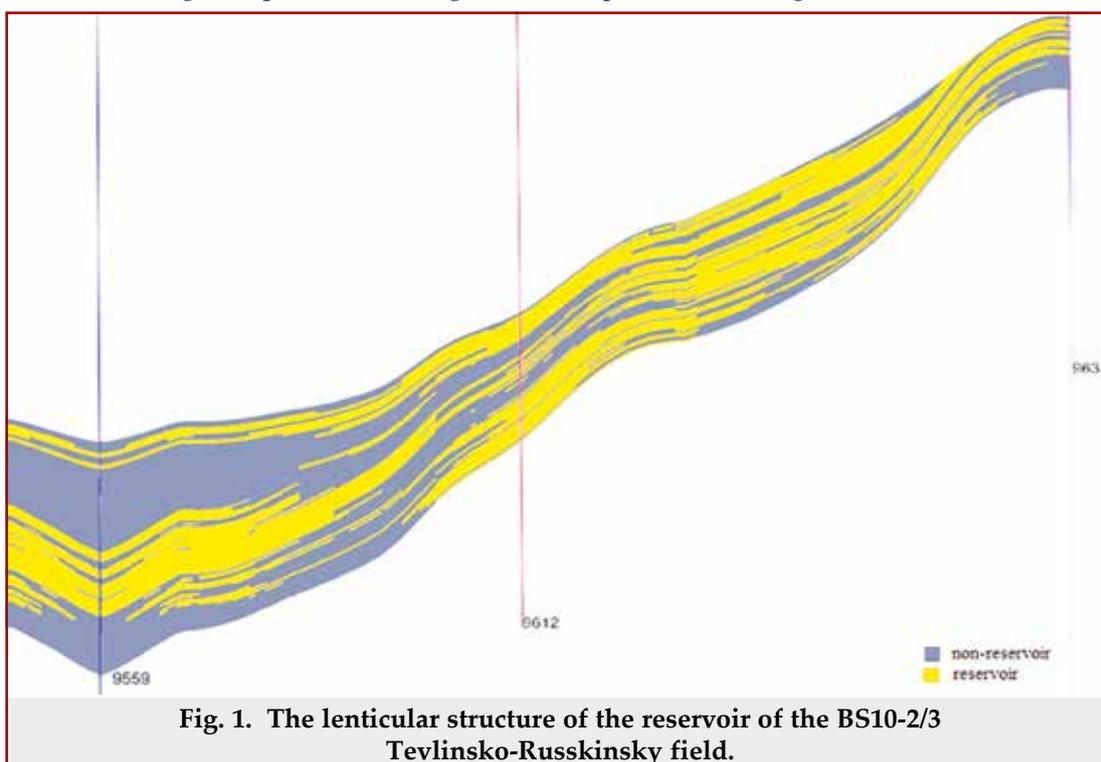
Fig. 1. The lenticular structure of the reservoir of the BS10-2/3 Tevlinsko-Russinsky field.
