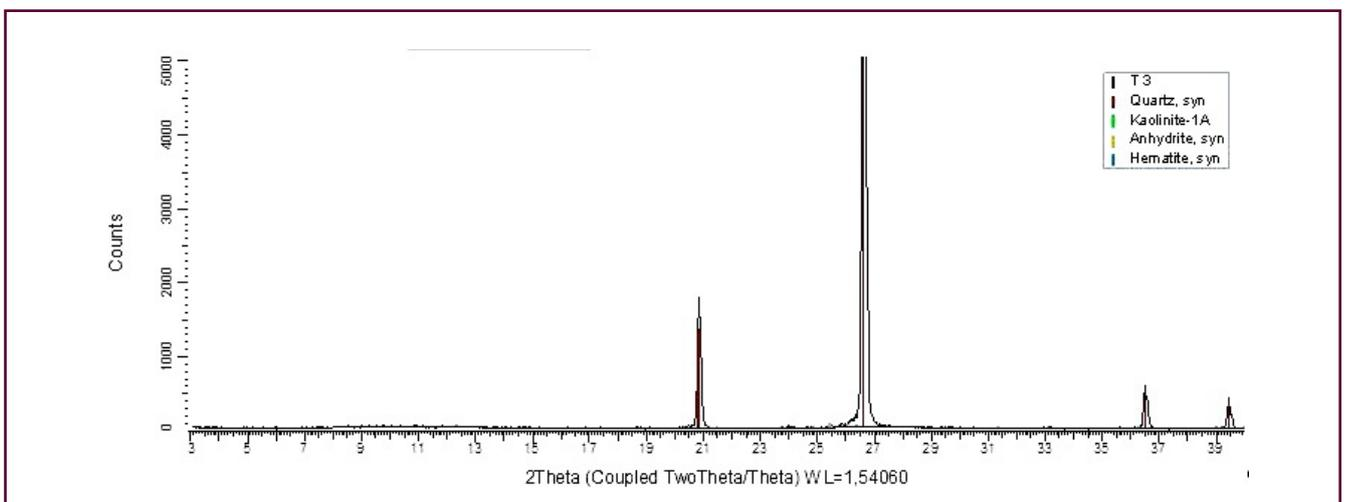
Fig.3. XRD spectrum of rock sample (T3) after combustion
