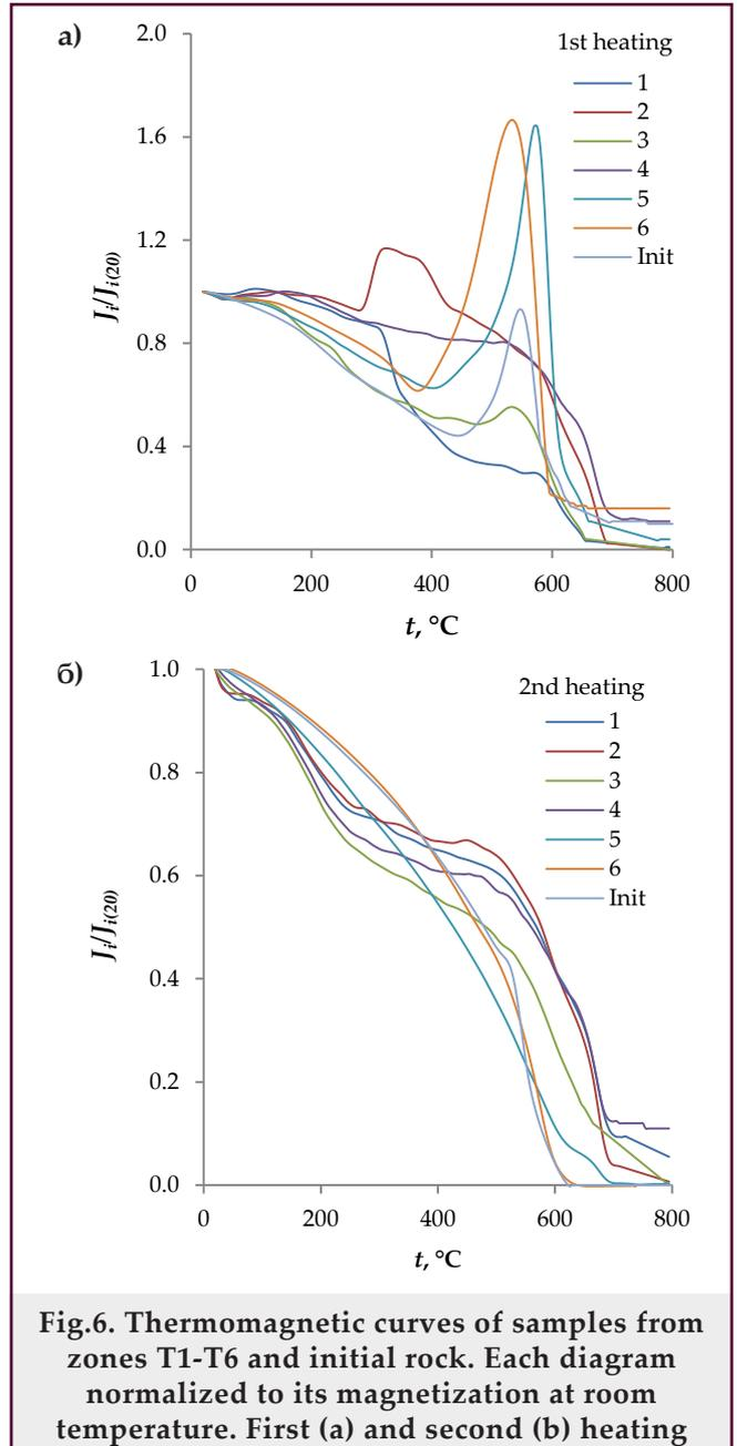
**Fig.6. Thermomagnetic curves of samples from zones T1-T6 and initial rock. Each diagram normalized to its magnetization at room temperature. First (a) and second (b) heating**
