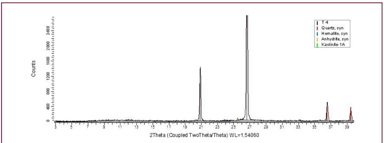
Fig.4. XRD spectrum of rock sample (T4) after combustion
