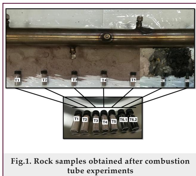
Fig.1. Rock samples obtained after combustion tube experiments
