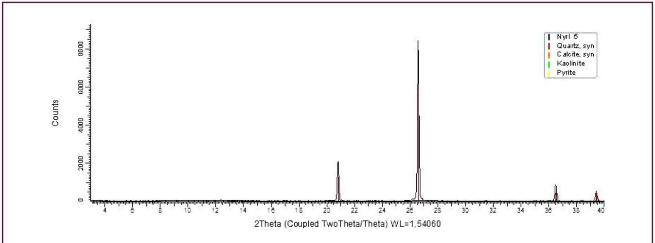
Fig.2. XRD spectrum of initial rock sample before combustion
