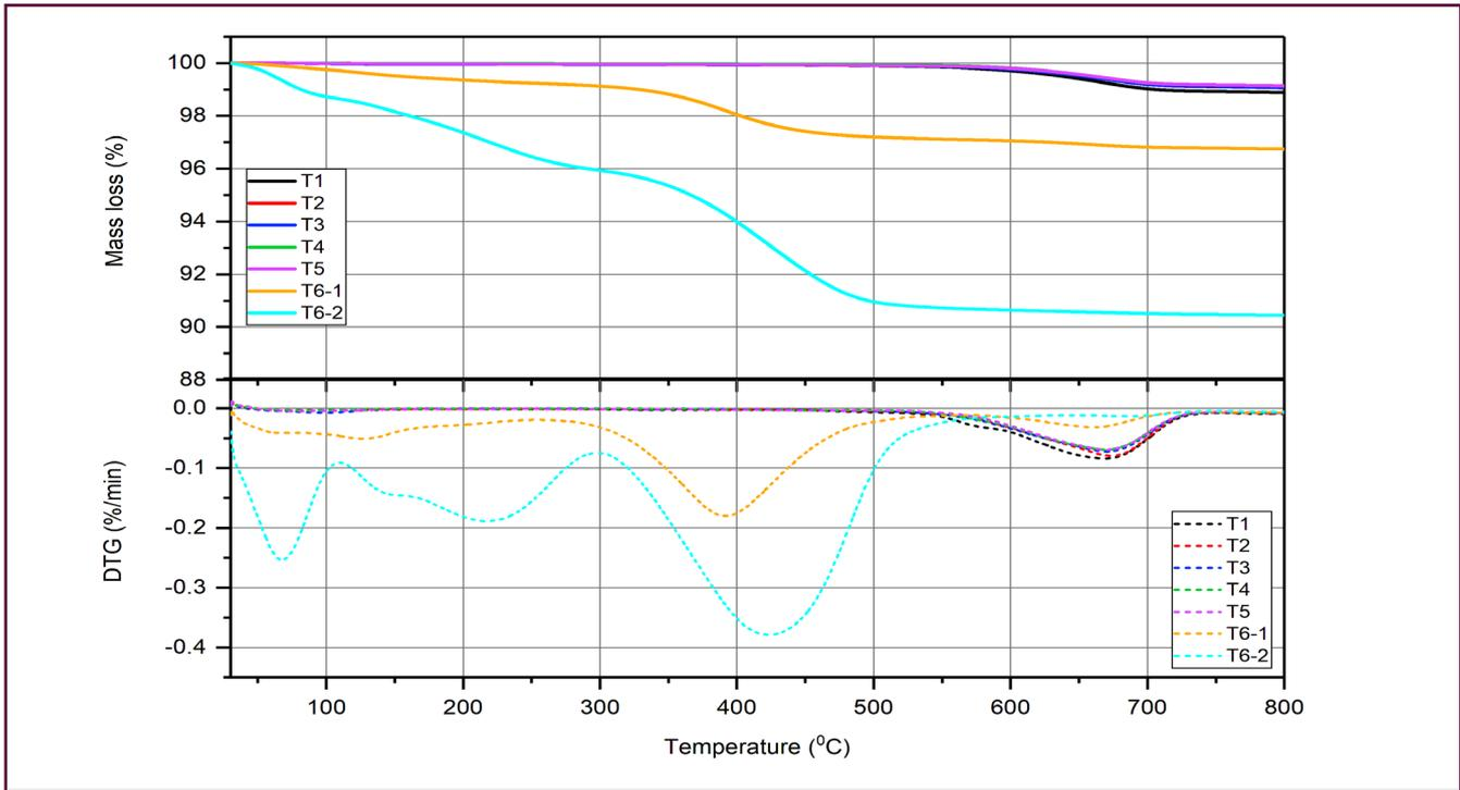
Fig.5. TG/DTG curves of samples T1, T2, T3, T4, T5, T6.1, and T6.2
