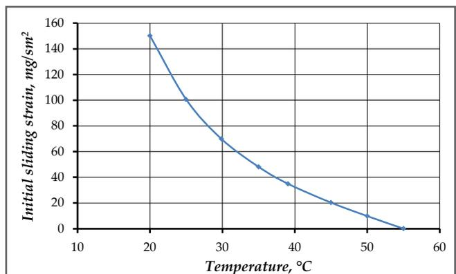
**Fig. 2. Oil initial sliding strain dependence from temperature**
