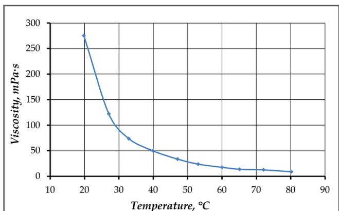
**Fig.3. Oil viscosity dependence from temperature**
