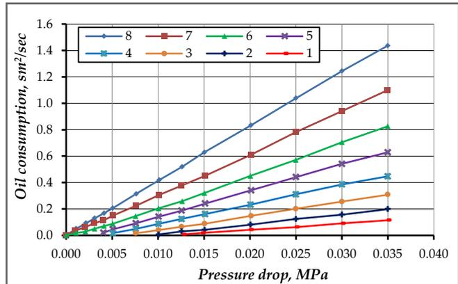
**Fig.1. Dependence of liquid consumption flowing through capillary under different temperatures from pressure drop**
