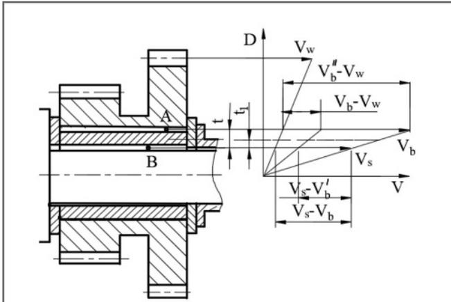
Fig. 4. The speed plan of the friction pairs located on the drive shaft
