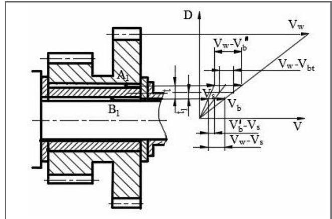
Fig. 5. The speed plan of the friction pairs located on the driven shaft
