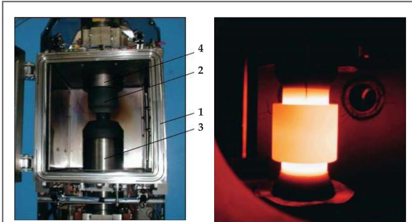
Fig. 1. View of the vacuum chamber of the Spark Plasma Sintering (SPS) device [4] 1 - vacuum chamber body, 2 - press-mold made of graphite, 3 - lower punch, 4 - upper punch
