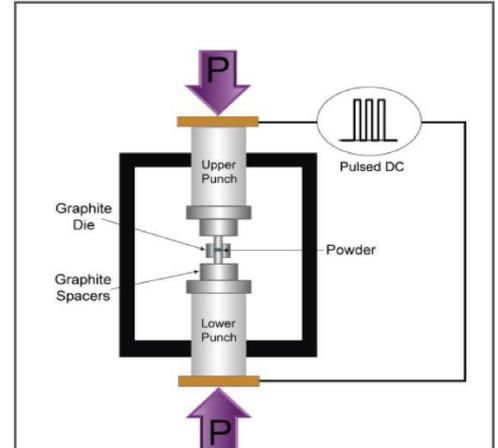
Fig. 2. Schematic diagram of the SPS apparatus [4]
