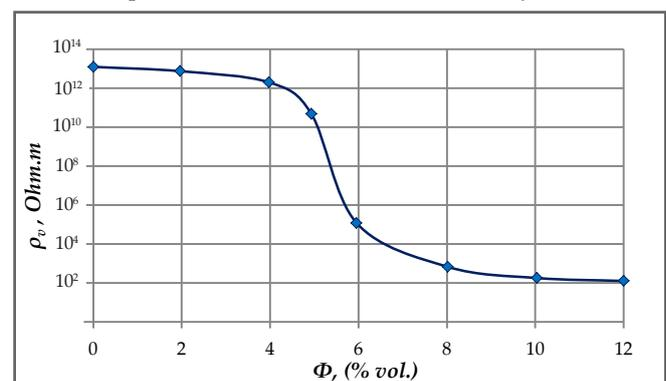
Fig. 3. Dependence of  $\rho_v$  on graphite concentration for PVC+Gr composites
