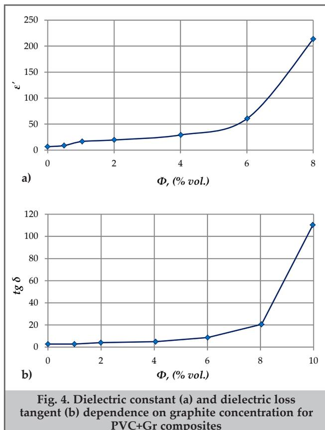
Fig. 4. Dielectric constant (a) and dielectric loss tangent (b) dependence on graphite concentration for PVC+Gr composites
