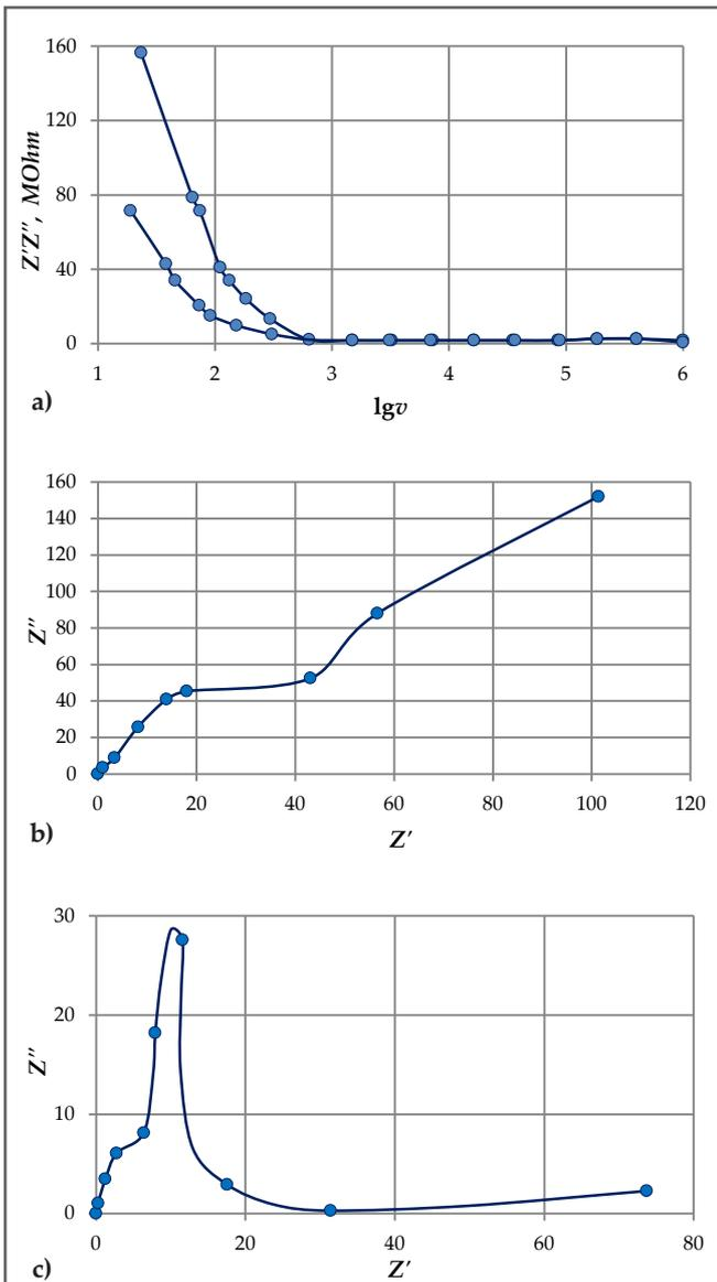
Fig. 2. Frequency dependences of the parameters  $Z'$  and  $Z''$  (a) and Nyquist diagrams for samples of F2ME (b) and F2ME+10% PKR-3M (c)
