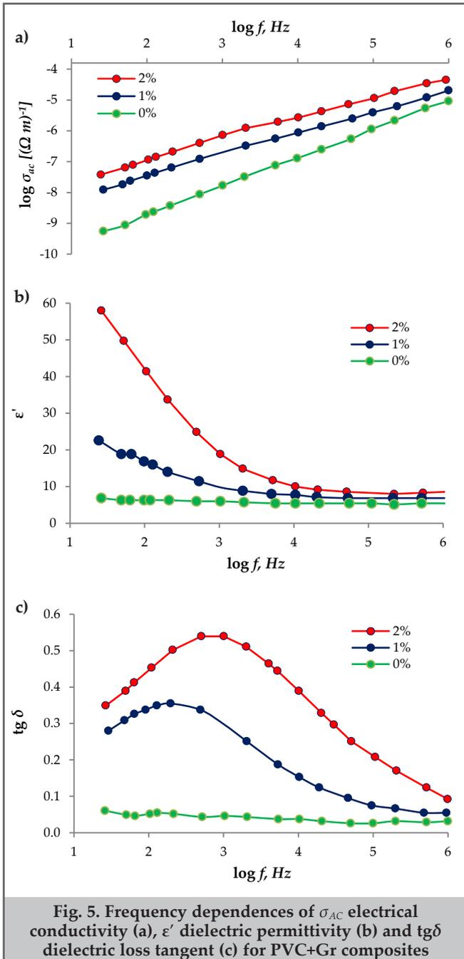
**Fig. 5. Frequency dependences of  $\sigma_{AC}$  electrical conductivity (a),  $\epsilon'$  dielectric permittivity (b) and  $\text{tg}\delta$  dielectric loss tangent (c) for PVC+Gr composites**
