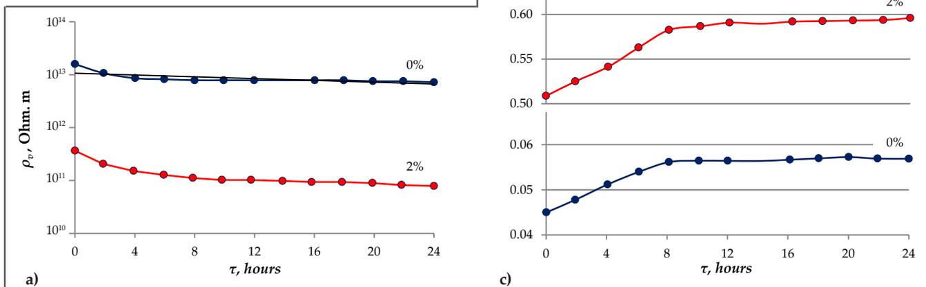
Fig. 9. Dependence of  $\rho_v$  (a),  $\varepsilon'$  (b) and  $\text{tg}\delta$  (c) on water retention time  $\tau$  for PVC and PVC+2%Gr composite
