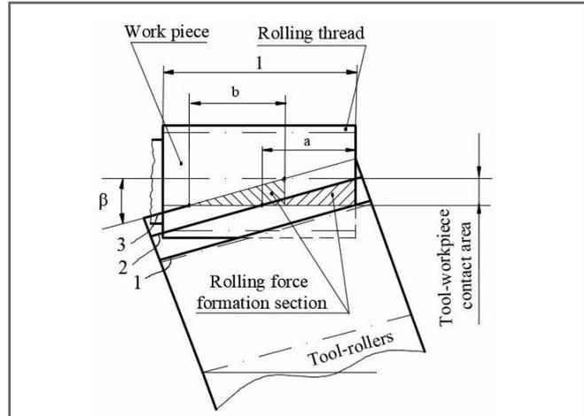
Fig. 4. Diagram of the fields of action of the rolling force when rolling a thread with an improved head
