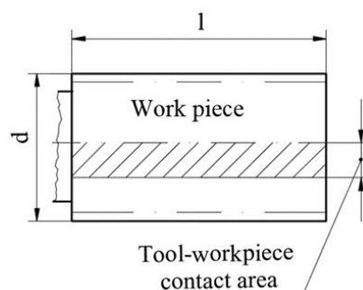
Fig. 1. Scheme of the fields of action of the rolling force when rolling threads by traditional methods
