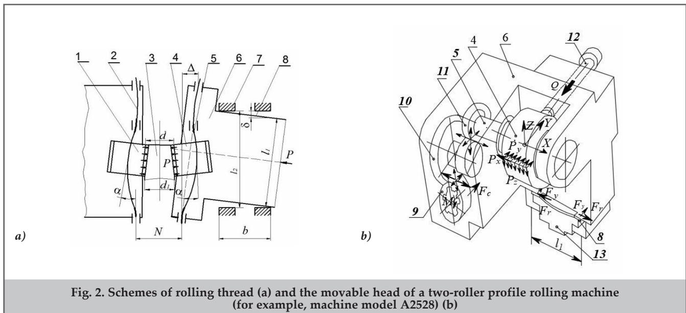
Fig. 2. Schemes of rolling thread (a) and the movable head of a two-roller profile rolling machine (for example, machine model A2528) (b)
