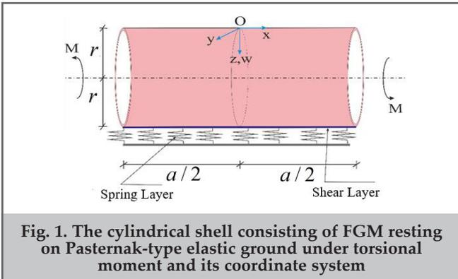
Fig. 1. The cylindrical shell consisting of FGM resting on Pasternak-type elastic ground under torsional moment and its coordinate system
