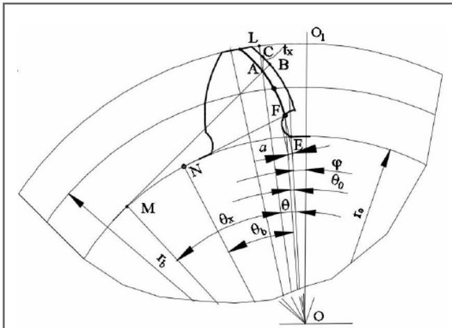
**Fig.4. Scheme of formation of the actual depth of cut when grinding the teeth (with rounding of the beginning of the profile) by copying**
