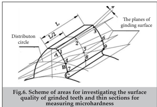
**Fig.6. Scheme of areas for investigating the surface quality of grinded teeth and thin sections for measuring microhardness**
