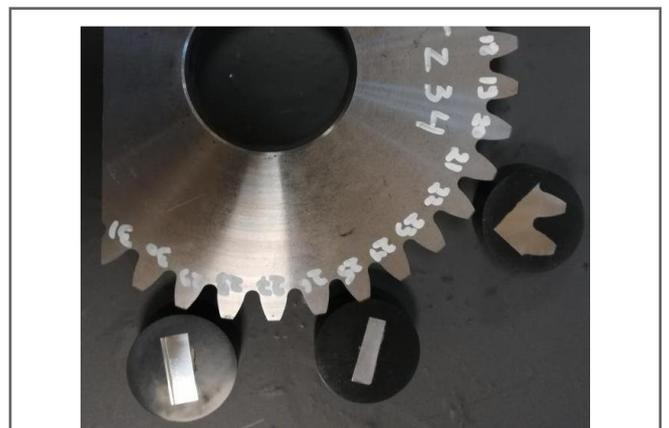
**Fig.5. Scheme of areas for investigating the surface quality of grinded teeth and thin sections for measuring microhardness**
