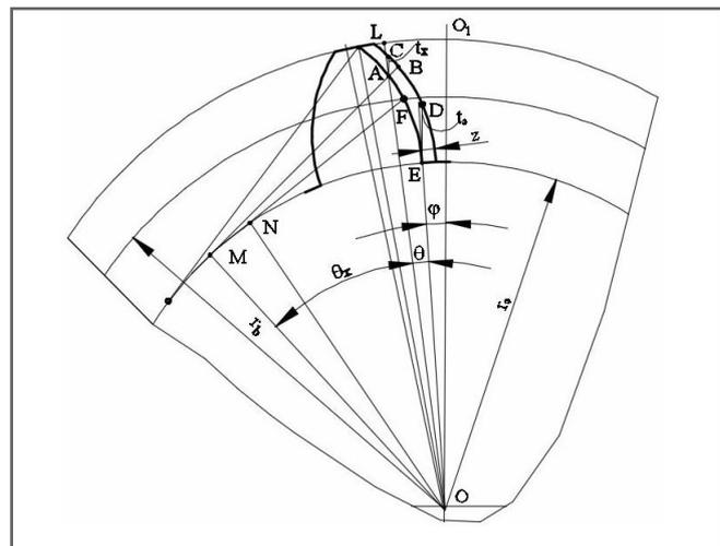
**Fig.3. Scheme of formation of the actual depth of cut in the grinding of teeth by copying**
