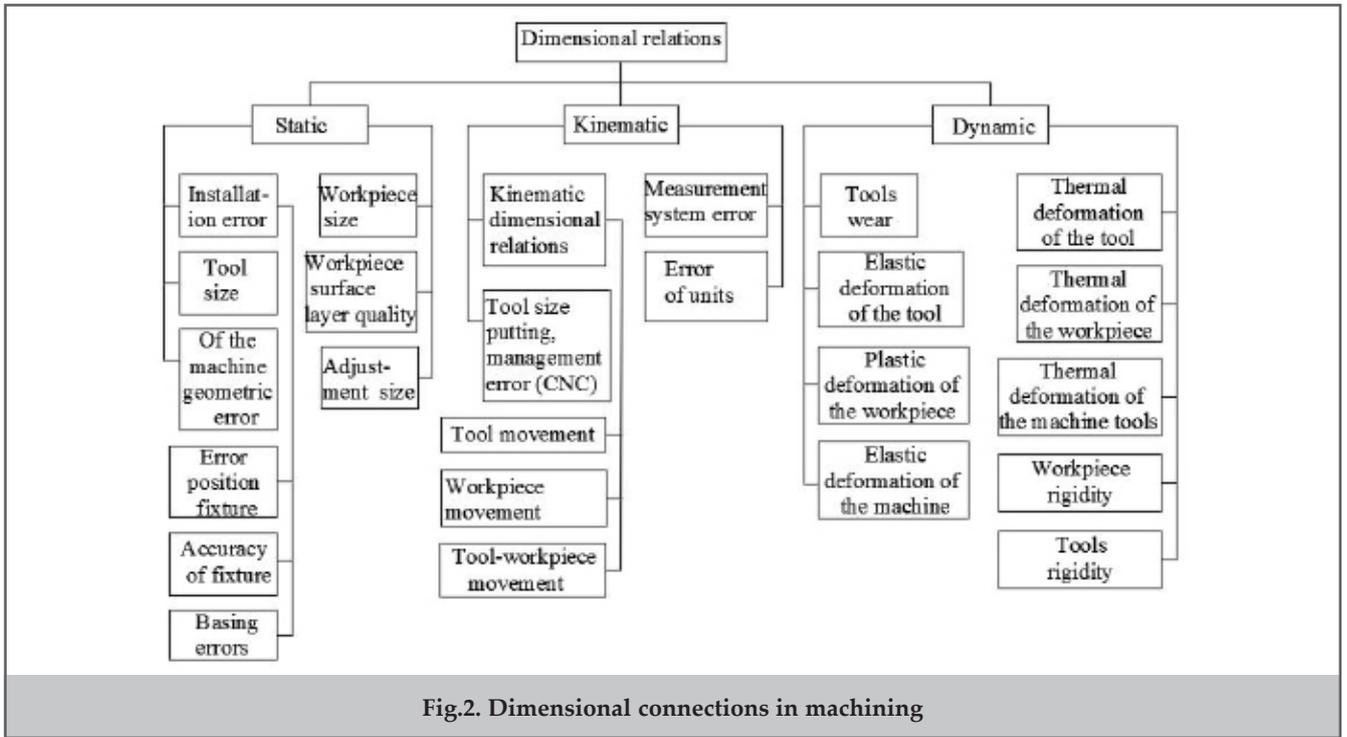
Fig.2. Dimensional connections in machining
