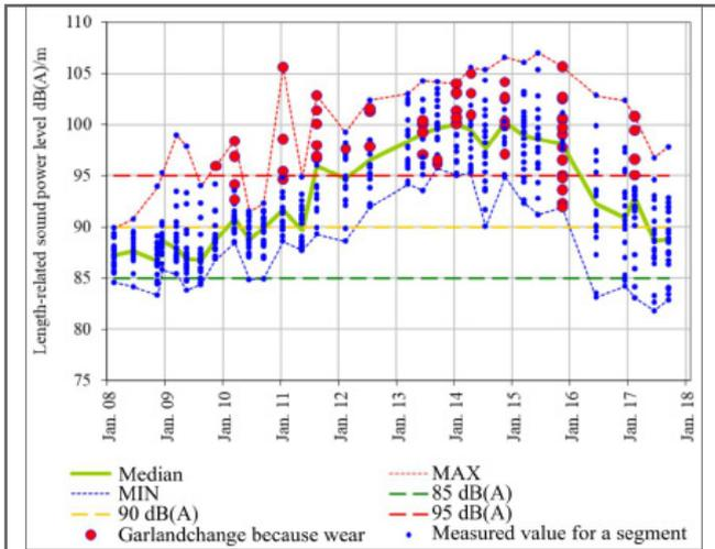
**Fig.3. Test results for test section 1, garland type A3G-2000-A159×750/600/750-10-5-18-Ü, maximum runout 0.5 mm, idler manufacturer A, test section with 20 segments and approx. 100 garlands**
