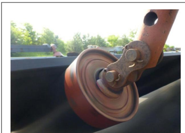
**Fig.4. Defective bearing seal on a support roller of manufacturer A, which subsequently leads to the penetration of contaminants into the rolling bearing, source: LEAG**
