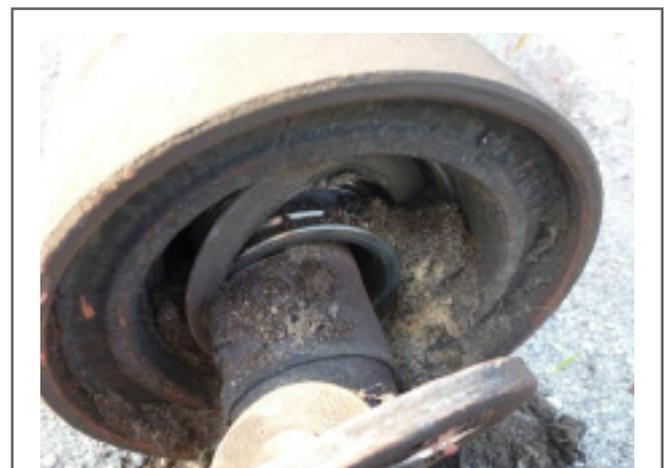
**Fig.5. Consequential damage to a support roller from manufacturer A in the form of a completely destroyed rolling bearing, the inner ring has already worked its way several millimetres into the support roller axle [1]**
