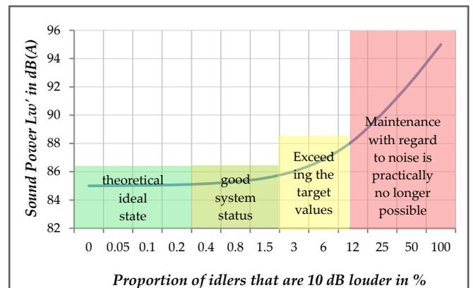
**Fig.1. Model calculation for the influence of damaged idlers on the average length-related sound power of a belt conveyor system with  $L_{w'} = 85$  dB(A) for undamaged idlers and  $L_{w'} = 95$  dB(A) for idlers with damaged idler bearings [13]**
