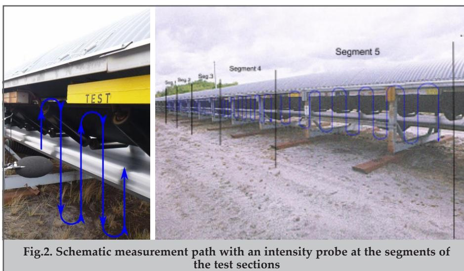
Fig.2. Schematic measurement path with an intensity probe at the segments of the test sections
