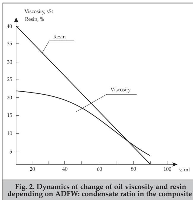
Fig. 2. Dynamics of change of oil viscosity and resin depending on ADFW: condensate ratio in the composite
