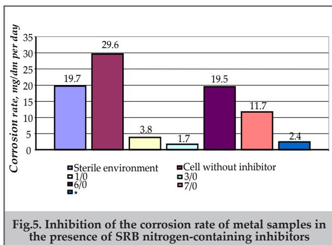
Fig.5. Inhibition of the corrosion rate of metal samples in the presence of SRB nitrogen-containing inhibitors
