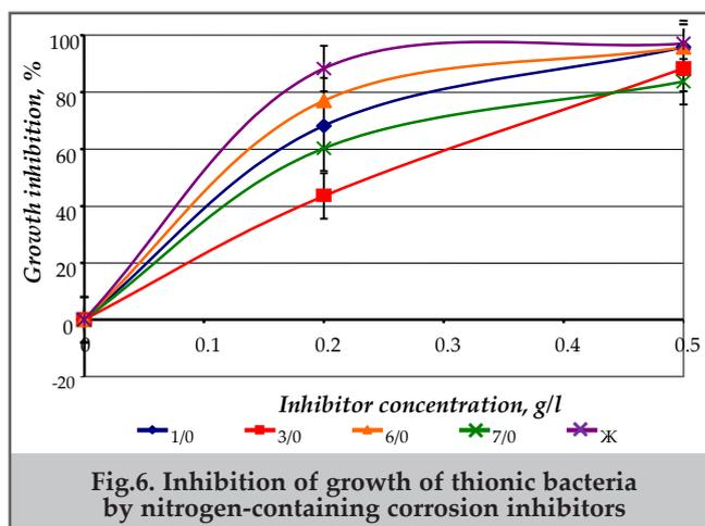
Fig.6. Inhibition of growth of thionic bacteria by nitrogen-containing corrosion inhibitors
