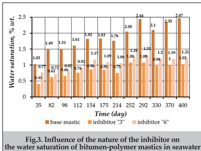
Fig.3. Influence of the nature of the inhibitor on the water saturation of bitumen-polymer mastics in seawater
