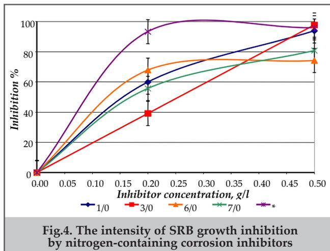
Fig.4. The intensity of SRB growth inhibition by nitrogen-containing corrosion inhibitors
